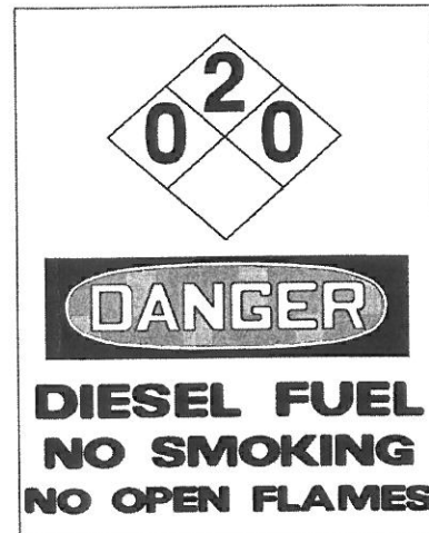
4 DANGER/TANK SIGNAGE A-4 NOT TO SCALE
